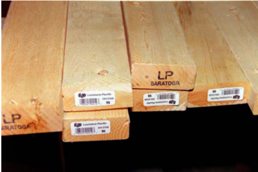
PHOTOGRAPH 3 2 x 4's USED IN FRAME CONSTRUCTION
