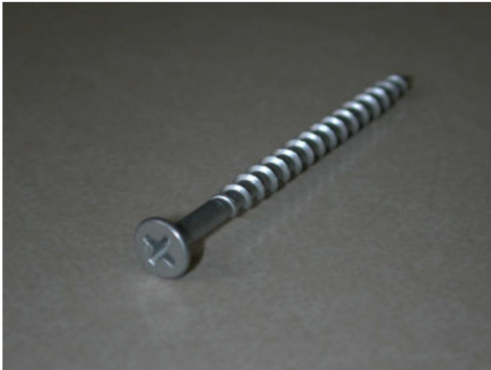
PHOTOGRAPH 8 2-1/2" GALVANIZED DECK SCREWS USED FOR PANELS 4, 5 AND 6
