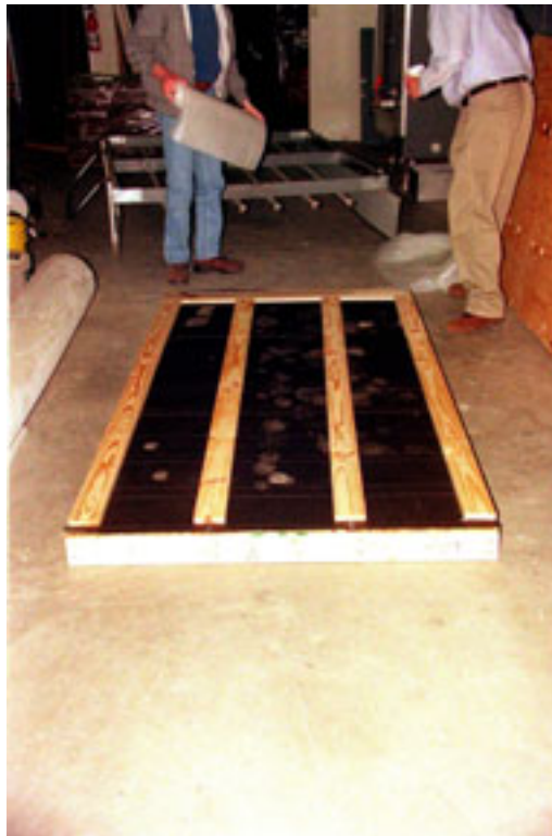
PHOTOGRAPH 12 FURRING STRIPS AND BASEBOARD ATTACHED TO FRAME
