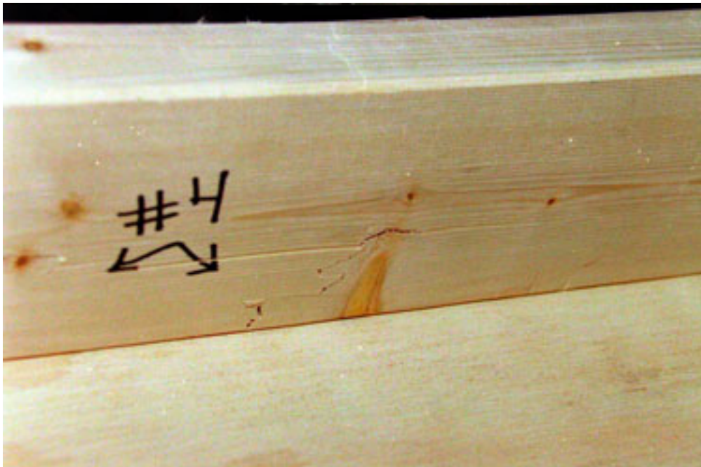
PHOTOGRAPH 26 SPECIMEN 4 FAILURE OF 2 x 4 STUD
