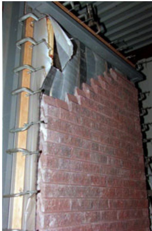
PHOTOGRAPH 28 BRICKS SEPARATED FROM PANEL AT FAILURE OF SPECIMEN 5
