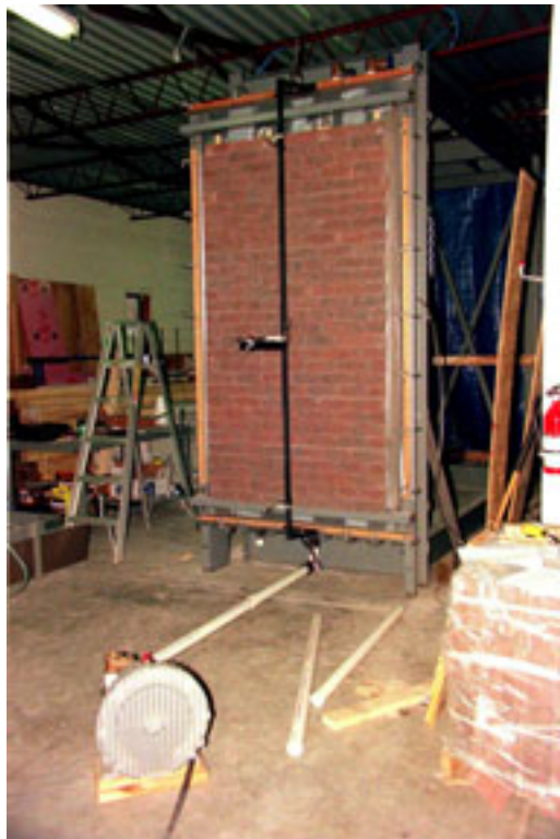
PHOTOGRAPH 18 COMPLETED NOVA BRIK WALL PANEL READY FOR TESTING
