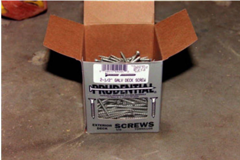
PHOTOGRAPH 7 2-1/2" GALVANIZED DECK SCREWS USED FOR PANELS 4, 5 AND 6
