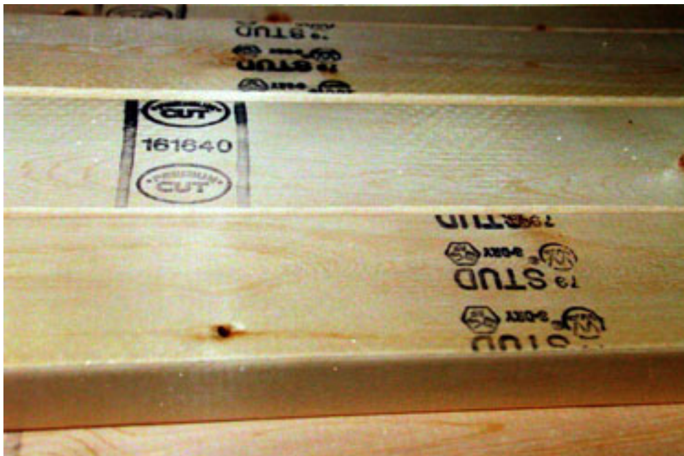
PHOTOGRAPH 4 2 x 4's USED IN FRAME CONSTRUCTION
