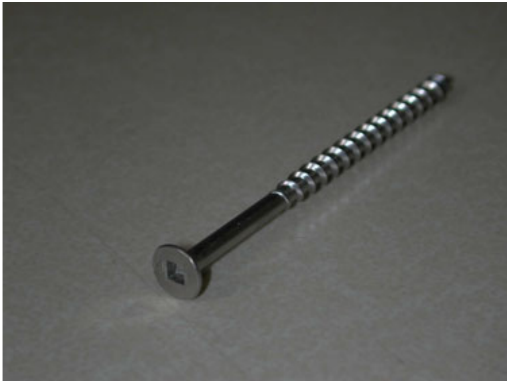
PHOTOGRAPH 6 #8 BY 3" STAINLESS STEEL BUNGE HEAD SCREWS FOR PANELS 1, 2 AND 3
