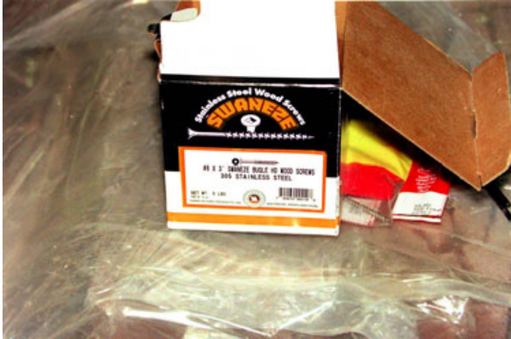
PHOTOGRAPH 5 #8 BY 3" STAINLESS STEEL BUNGE HEAD SCREWS FOR PANELS 1, 2 AND 3
