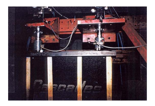
Photo 3 - Close-up view of hydraulic jacks
