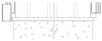
Position the starter strip's flange underneath the furring strips and assure a
