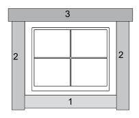
the waterproof membrane properly. Ensure that adhesive flashing is adequately bonded to the vapor/air barrier and in full contact with the perimeter surface opening.
