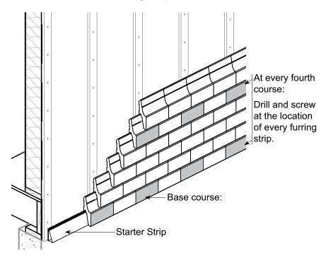
Note: Use #8 or #10 corrosion-resistant screws to fasten furring strips to the studs. Make sure the screws penetrate at least 1 1/4" (32mm) into the studs.
