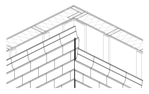
COVER THE CORNER WITH HOUSEWRAP OR WITH A SELF ADHESIVE WATERPROOF MEMBRANE. INSTALL 1"X6" (19MM X 140MM) BOARDS OVER THE CORNER. INSTALL NOVABRIK ON ONE WALL ALL THE WAY TO THE CORNER, WHILE INSTALLING THE ADJOINING WALL, LAY A CORD OF BACKER-ROD UP THE BRICK WALL. CUT AND ATTACH END PIECES TO ACHIEVE A CONSISTENT 3/8" (10MM) GAP
