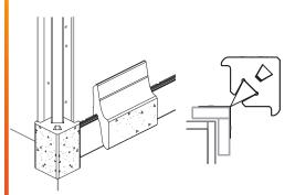
3 - SLIDE DOWN THE FIRST CORNER BLOCK AND ALIGN WITH THE FIRST COURSE OF NOVABRIK. FASTEN INTO CORNER STRIP WITH ONE SELF-TAPPING CORROSION RESISTANCE SCREWS.
