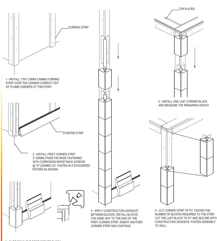
3 - SLIDE DOWN THE FIRST CORNER BLOCK AND ALIGN WITH THE FIRST COURSE OF NOVABRIK. FASTEN INTO CORNER STRIP WITH ONE SELF-TAPPING CORROSION RESISTANCE SCREWS.
