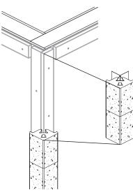
6 - CUT CORNER STRIP TO FIT. FASTEN THE NUMBER OF BLOCKS REQUIRED TO THE STRIP. CUT THE LAST BLOCK TO FIT AND SECURE WITH CONSTRUCTION ADHESIVE. FASTEN ASSEMBLY TO WALL.
