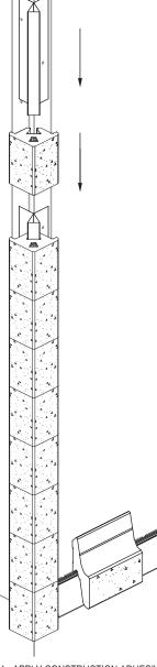
4 - APPLY CONSTRUCTION ADHESIVE BETWEEN BLOCKS. INSTALL BLOCKS THE SAME WAY TO THE END OF THE FIRST CORNER STRIP, INSERT ANOTHER CORNER STRIP AND CONTINUE.
