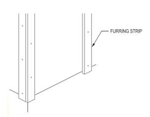
1 - INSTALL 1"X4" (19MM X 89MM) FURRING STRIPS OVER THE CORNER. CORRECT OUT OF PLUMB CORNERS AT THIS POINT.
